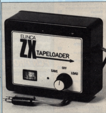
GO-BETWEEN — This device could mark the end of futile juggling with the volume control on your cassette recorder as you try to load a program on to a ZX81. Called the ZX Tape Loader, it sits between your cassette deck and your ZX81 and stabilises the signal in both directions. It should also make life easier when you're switching from LOAD to SAVE — with its three-way switch there will be no need to plug and unplug leads from the input and output sockets.
